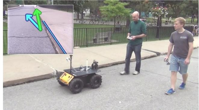
Fig. 1. Robot operator (left) collaborating with autonomous vehicle during boundary patrol field trial, supervised by experimenter (right). Inset: robot autonomy’s camera view (not shown during field trial), overlaid with detected boundary (blue line), autonomy’s steering command (blue arrow), and operator’s intervening command (green arrow).
